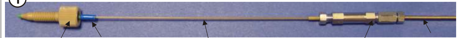
1 Column inlet: glass-PEEK capillary, 1/32" (0,8 mm) OD, direct connection to sample injector 1/16" (1,6 mm) OD
