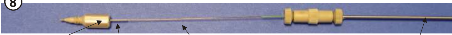
8 Column inlet: fused silica capillary, 360 µm OD, direct connenction to sample injector 1/32" (0,8 mm) OD
